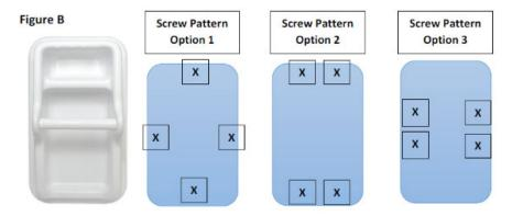
Step 3: Drill 4 mounting holes in the perimeter of the part. See diagram for hole location suggestions.
